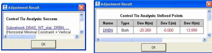
Figure 6-26. Control Tie Results – Successful and Not Successful Examples
