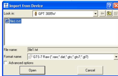
Figure 3-31. Import From Total Station
