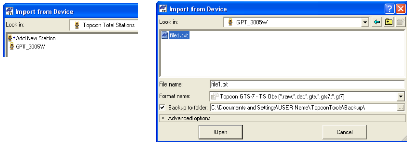
Figure 3-41. Import From Topcon Total Station
