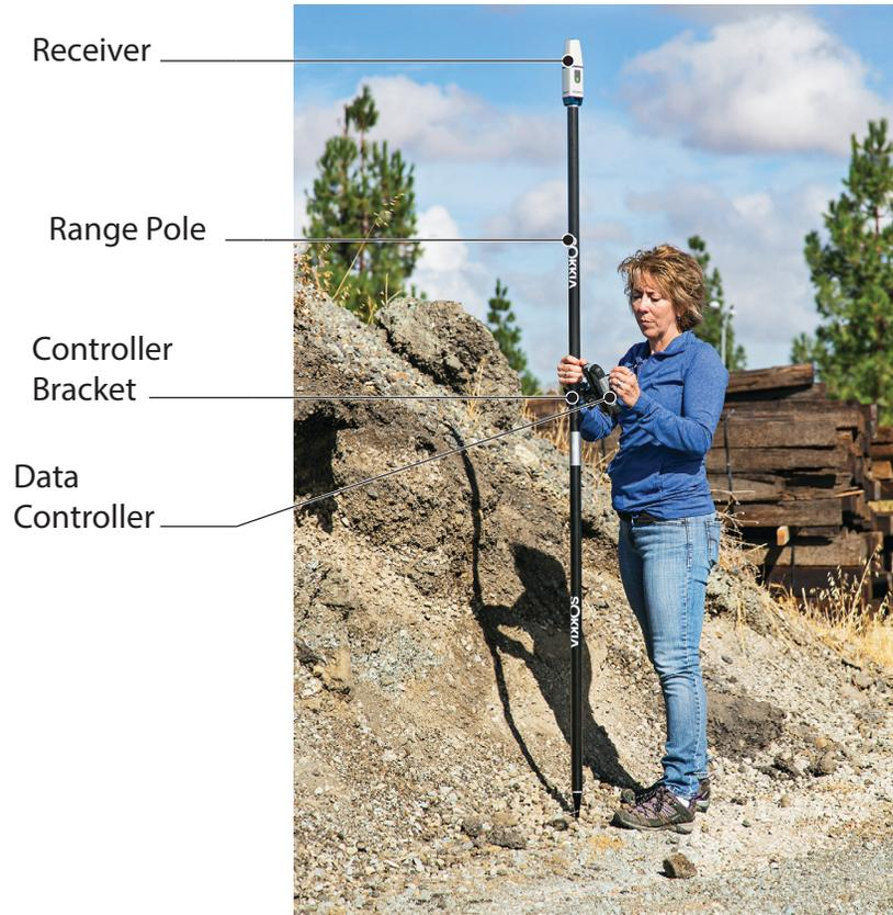
**Figure 20: RTK Rover**
