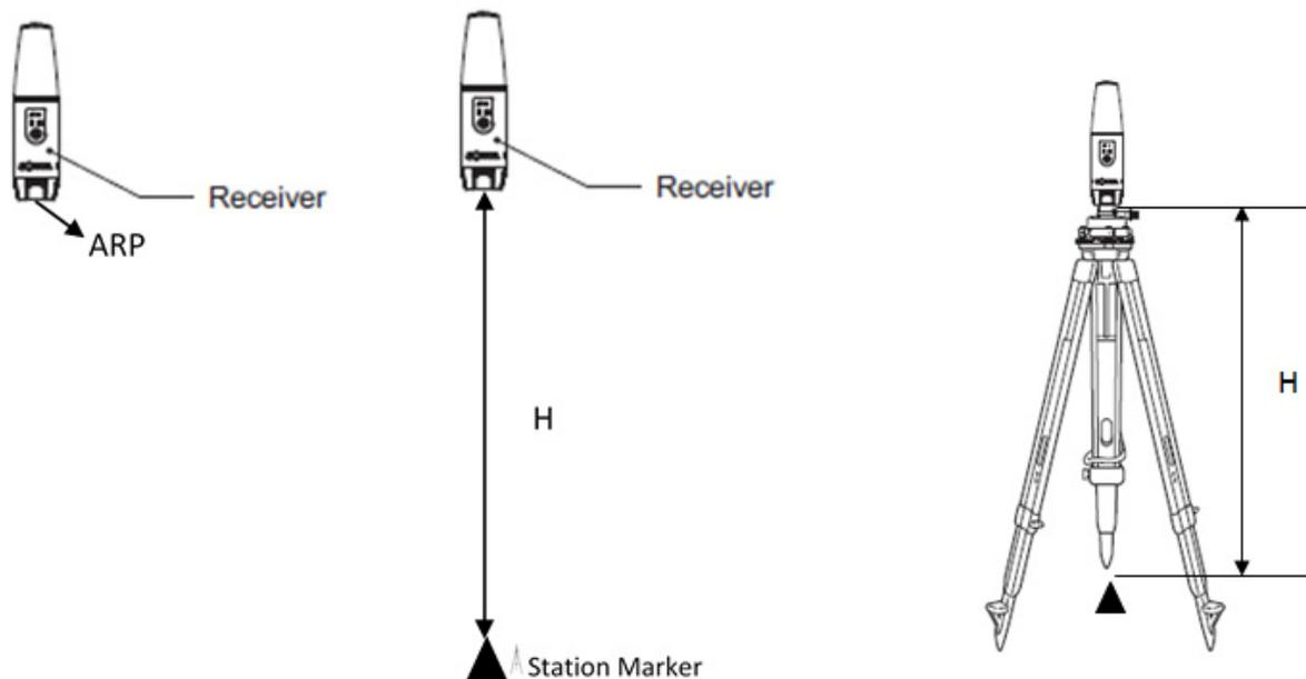
**Figure 21: Obtaining Antenna Height**
