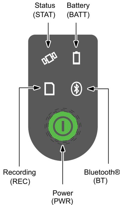
Figure 5: LED Display Panel
