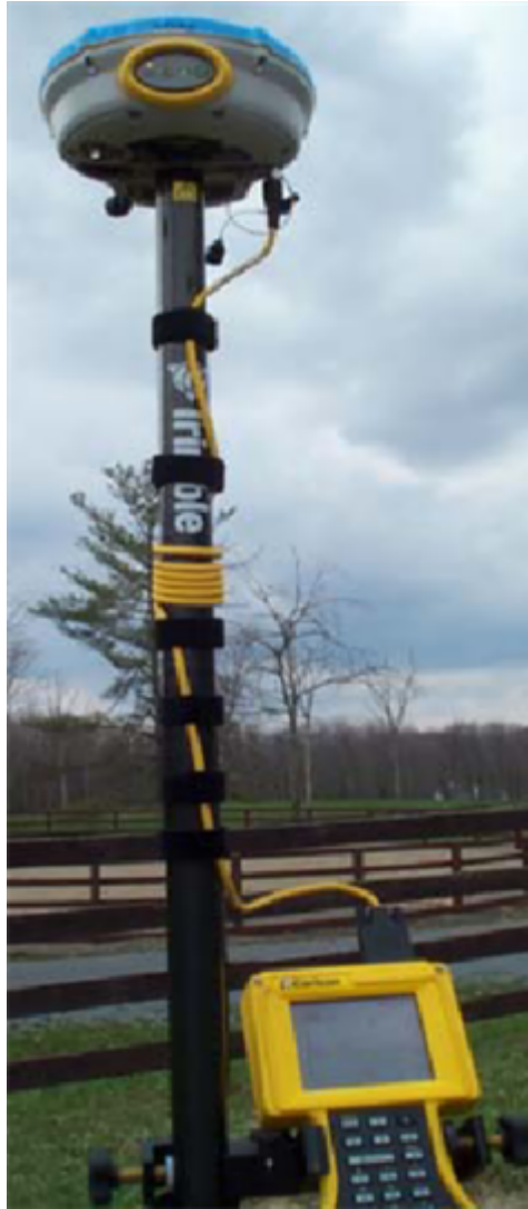
The Trimble 5800 with Zephyr antenna has a panel that includes an On-Off button at right.
